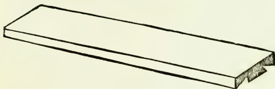
Fig. 47.—RIDGE BOARD OF COVER.
