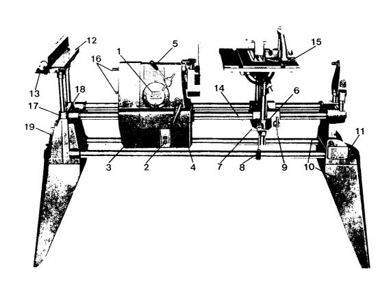
This 5-in-one unit would be ideal for the commercial beekeeper or home handyman. It has a 250 mm blade, a 300 mm disc sander, an 860 mm lathe, a verticle drill press and a horizontal drill press, all driven by a 2 speed  $l_2$  h.p. motor.
