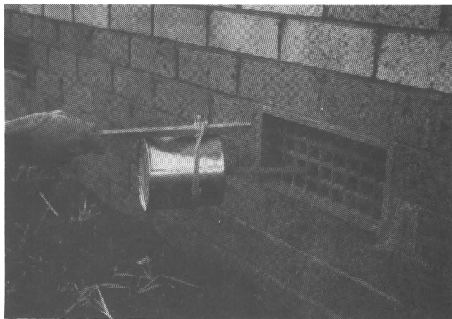
Fig. 3: An insecticide smoke applicator in use against a colony located under a house.
