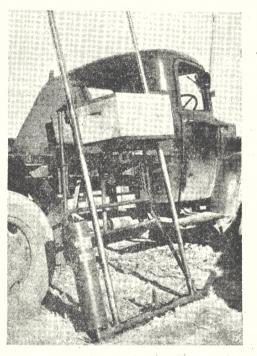
Operating on a tank of compressed air this machine is not reliant on any other means of power. The only maintenance required is a few drops of oil daily when in use.
