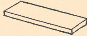
Fig. 3. Length 14 \frac{1}{4} " x 4 \frac{1}{2} " wide x 3/8" deep. Bevel slightly to give downward slope.
