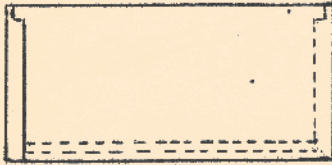
Fig. A. Wet cappings are placed in box. Wire netting on frame is at base. Wire held by cleats.
