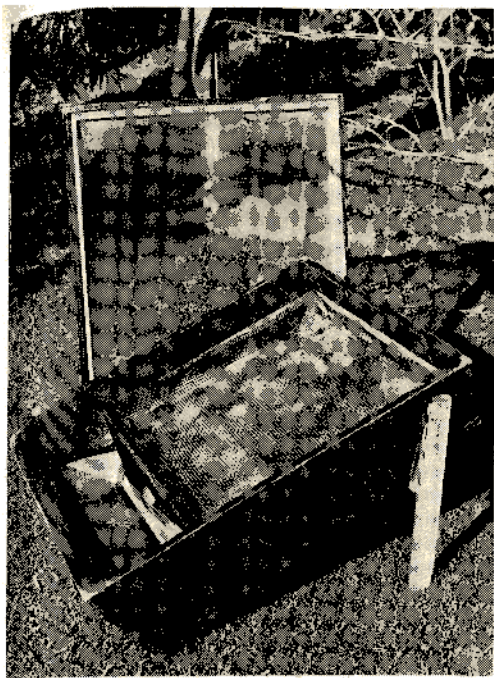
Fig. 3. Solar extractor with lid raised showing components in position.
