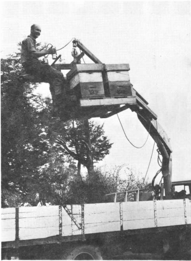
John Syme (Staveley) using the Mark I forks with the controls mounted on the forks. John plans to change the design of the pallets to load from the ends.
