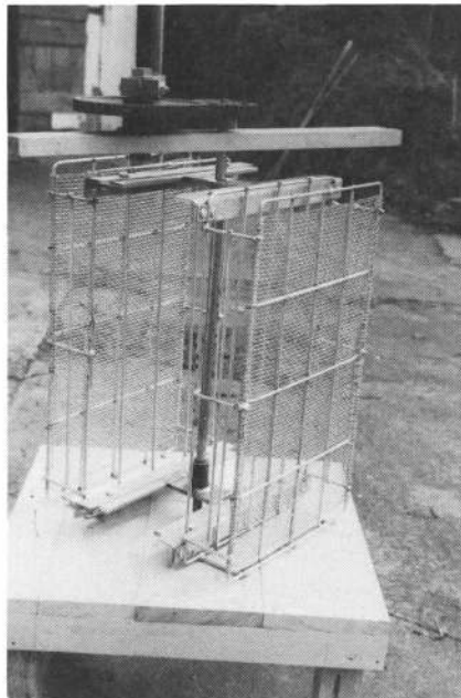
Nathan. The fixed baskets from the extractor. The combs must be lifted out and reversed by hand.
