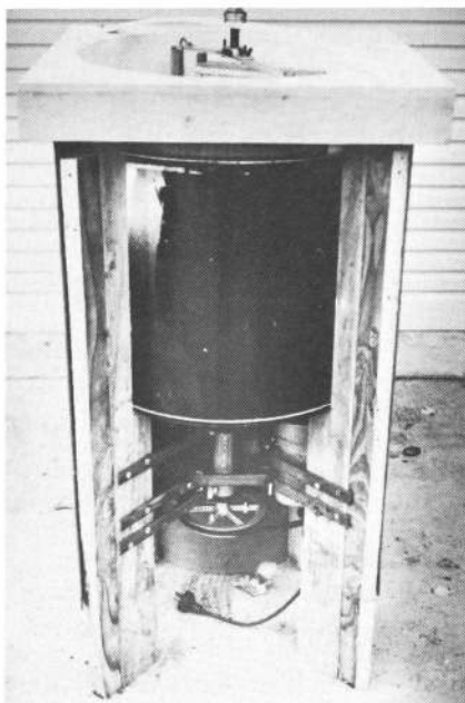
Salisbury: general view of the bottom drive extractor with the sump tank.
