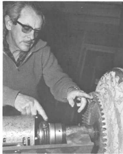
Robert Davidson comparing his own gearing system (left), to the original (right) concrete mixer gearing system.
