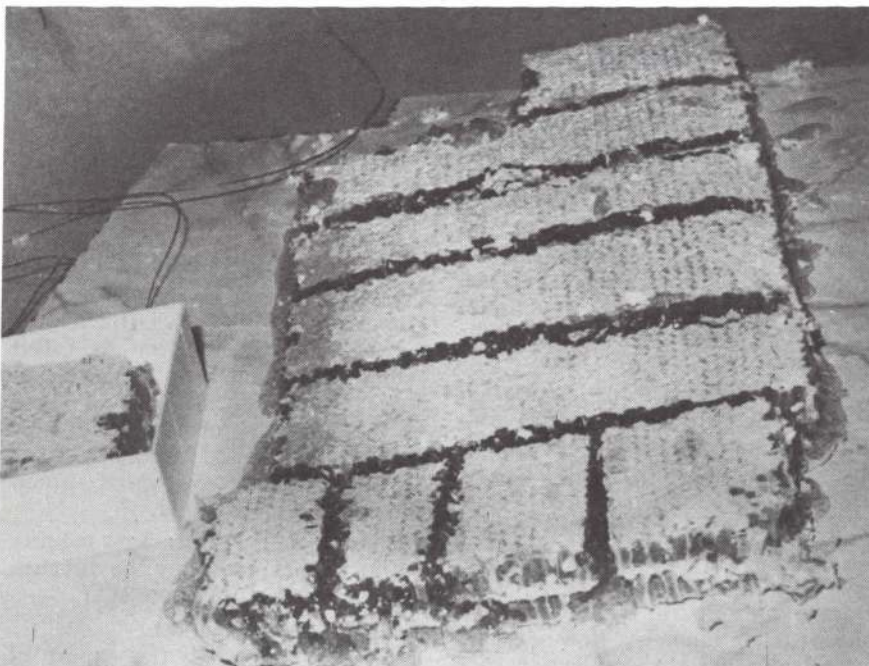
Cut up to size wanted – a cold sharp knife will do. Cutting on formica will reduce the mess.
