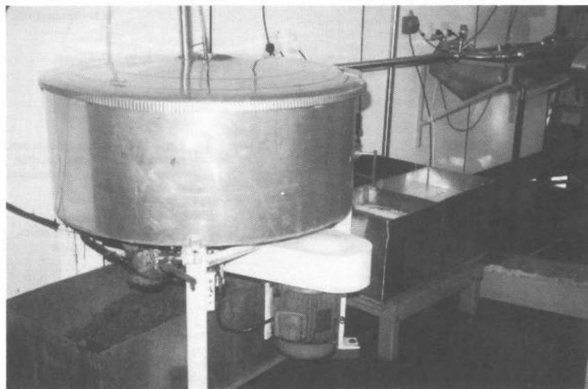
Figure 3: A centrifuge. Wax is deposited in the tray beneath the machine, and honey is run out into the baffle tank to the right.
