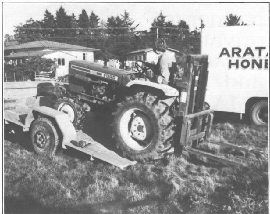
Larger outfits are better able to justify the expense of equipment such as forklifts. This four-wheel-drive forklift and tip trailer is used by Arataki Honey in Hawke's Bay, for shifting hives and for working the hives in wet apiaries.
