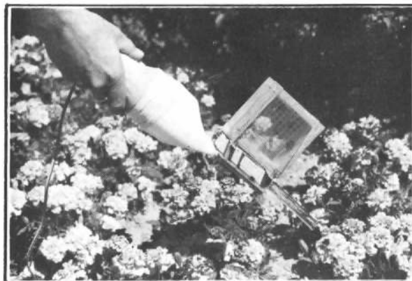
This bee collector was invented by Pat and gathers bees by sucking them into the cage.
