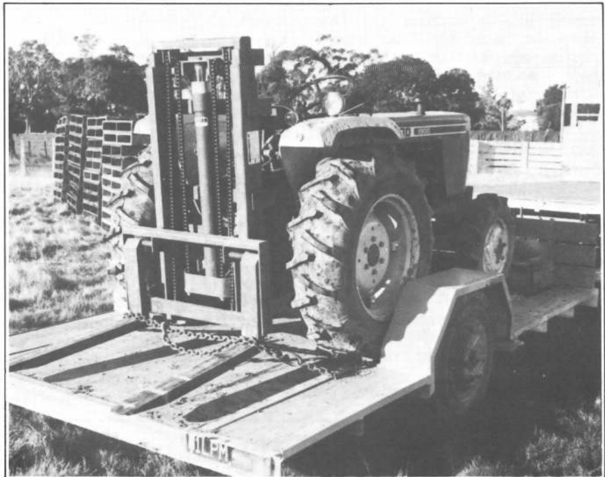
Larger outfits are better able to justify the expense of equipment such as forklifts. This four-wheel-drive forklift and tip trailer is used by Arataki Honey in Hawke's Bay, for shifting hives and for working the hives in wet apiaries.
