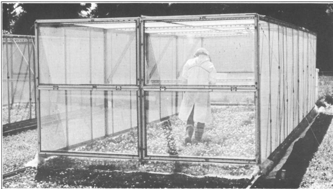
The "cage". This is the most common method of first testing insecticides in the field. A single storey hive is placed inside this structure and the bees left to tend the sprayed white clover inside.
