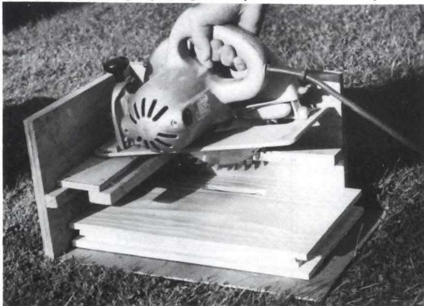
Figure Two: Putting in the handholds.
