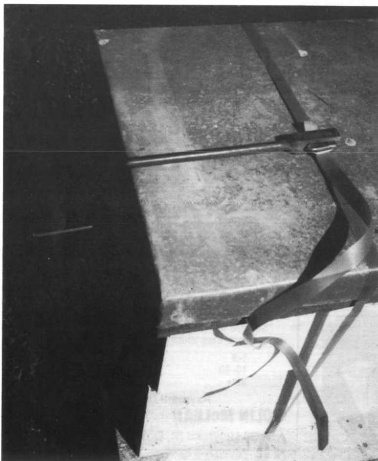
Above: The strap is tight enough to prevent it being removed by fingers alone. Below: The mouth of the crank is inserted over the wire buckle.
