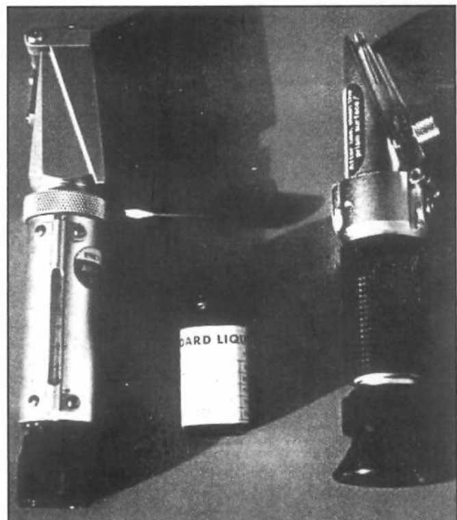
Fig. 1 - Two common models of hand-held refractometers used to determine the moisture level in honey. The older model is the one on the left.
