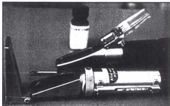
Fig. 2 - Hand-held refractometers with the hinged prisms open showing where a drop of honey is placed when measuring the moisture level of honey and where the test glass or fluid is placed for calibrating the instruments.
