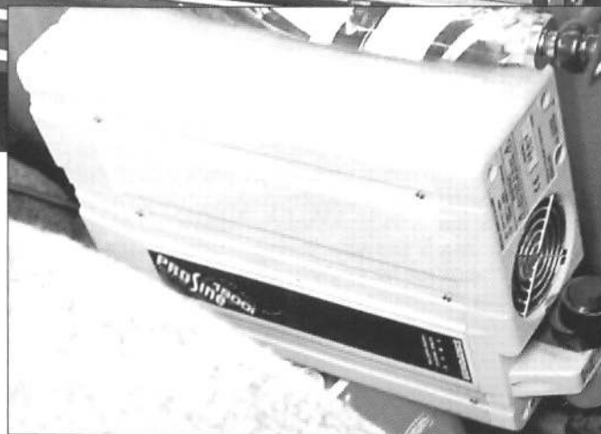
Sugar feeding set-up, with 12/230 volt inventor and double battery set-up.
