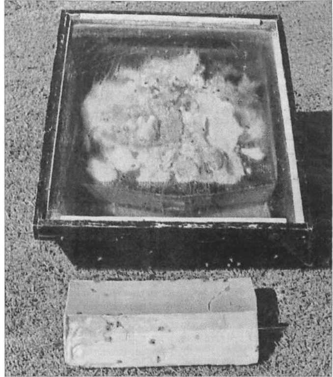
Solar wax extractor in use. In the foreground is a block of wax previously melted.
