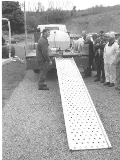
Ramp set-up saves double handling for loading honey supers
