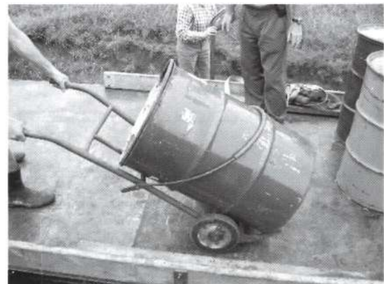
I noticed the drum barrow while assisting to unload drums at Gary Tweeddales. It was an old type used for open top drums that used a round bar to hold the drum on while transporting. Very safe, I thought, and better than the attachment that just locks into the top of the drum rim.
