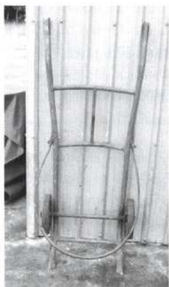
I noticed the drum barrow while assisting to unload drums at Gary Tweeddales. It was an old type used for open top drums that used a round bar to hold the drum on while transporting. Very safe, I thought, and better than the attachment that just locks into the top of the drum rim.
