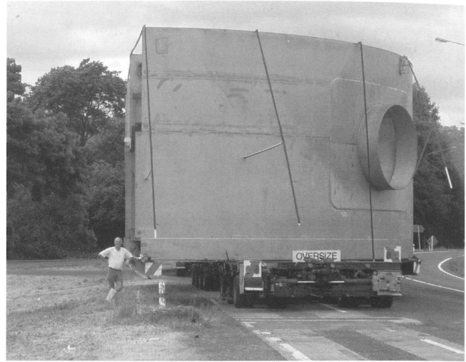
The silo took up both sides of the road from fog line to fog line, and scraped under the power lines with scoops.
