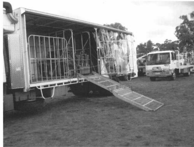
Trailer unit set up for moving bee hives, heat exchange for cooling plus fine mist sprayer.
