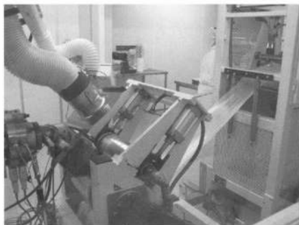
A ribbon of Apivar strips leaves the extruder.
