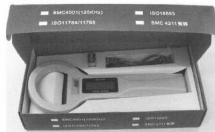
Example of an RFID hand-held reader.
