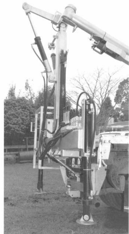
The boom can be locked in place above a load two hives high (four supers and two bases) or can be dropped to strap down on an empty deck as shown here.
