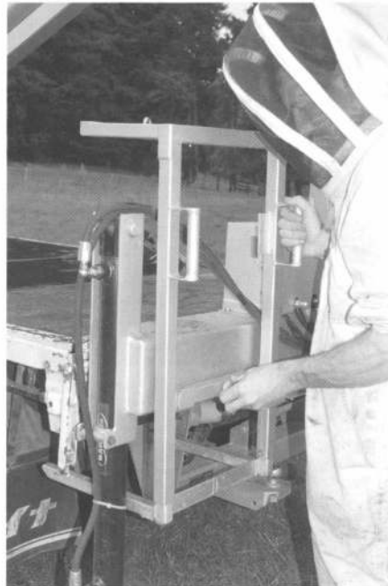
The cradle is locked into place on the truck for easy transport without taking up deck space.
