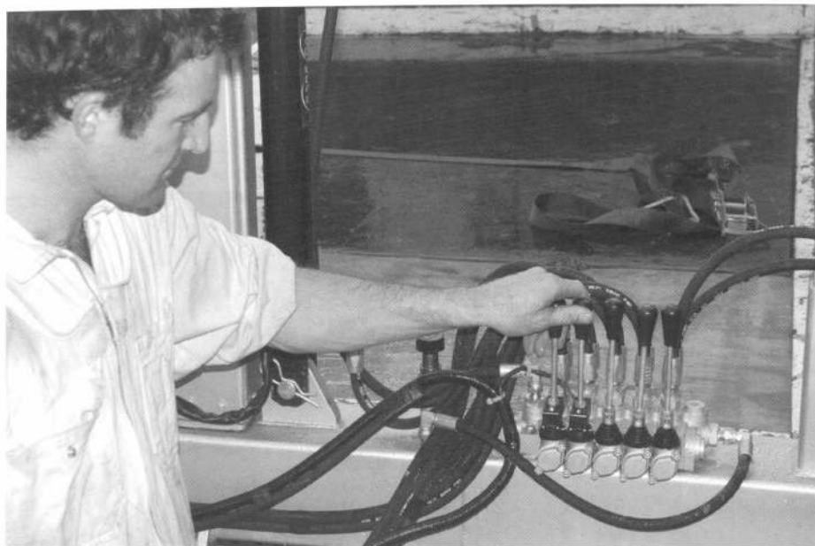
LED lights tell the operator which way to move in order to level the crane. When both lights on both levers go out, the crane is level. Photos: Kushla Haenen.
