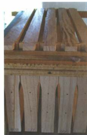
Hoffman frames sit in a jig awaiting wiring. Note the bee space gap between the top bars, which allow the bees to move up through the hive, and also between the sides and bottoms of the frames.
