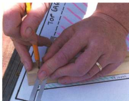
Lining up sidebars on the template to mark the required angle to be cut.
