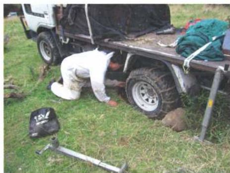
From left to right: Truck jacked up. After the second lift: chains and more stones applied. Ready to roll with David as a counterweight. Photos: Frank Lindsay.
