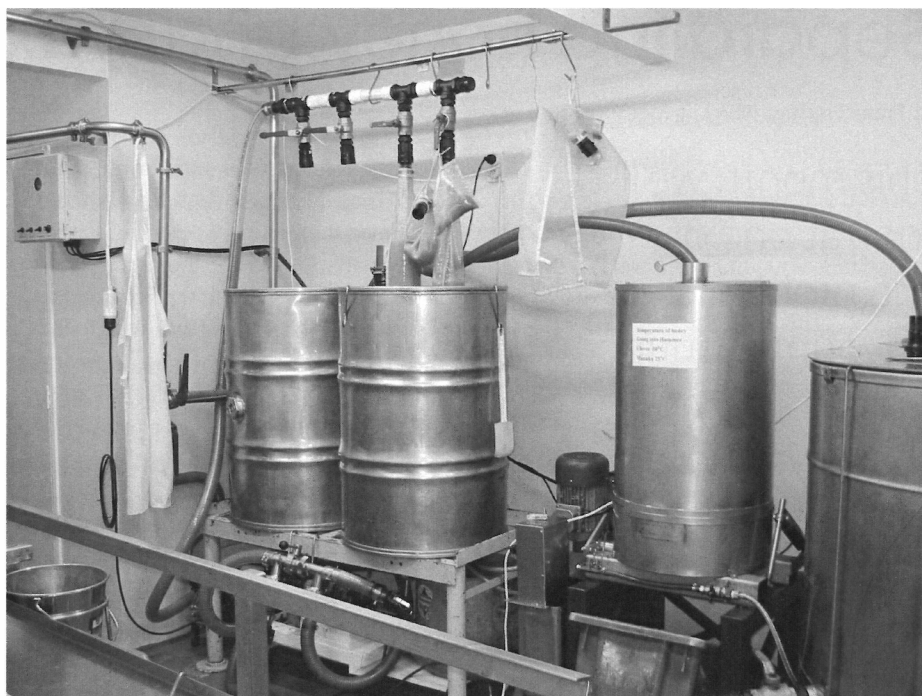
My honey house in 2010. The 'hummer' (old model) spinner is on the right with the final filtering system over the tanks. The looping pipes at the front are now tucked underneath. I run the first 60 kg through and then bypass the filters as the wax in the hummer acts as a filter and use the filters again during the dump, which drains the last of the honey from the hummer at the end of the day. Photos: Frank Lindsay.
