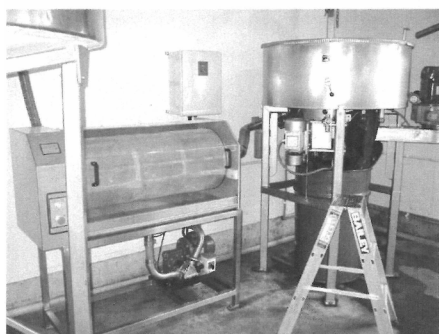
A rotary honey strainer produced by Peter Boutelje. This photo was taken in Don Tweeddale's honey house.
