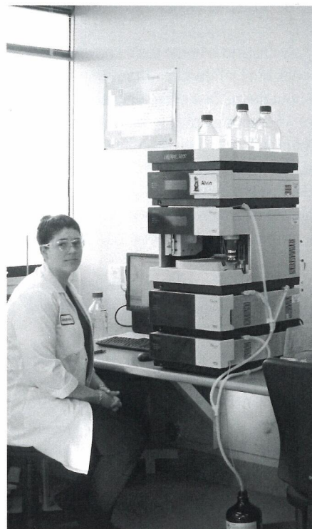
Hill Laboratories team leader Ashleigh Jacques with the new Ultra Performance Liquid Chromatography instrument (UPLC).
