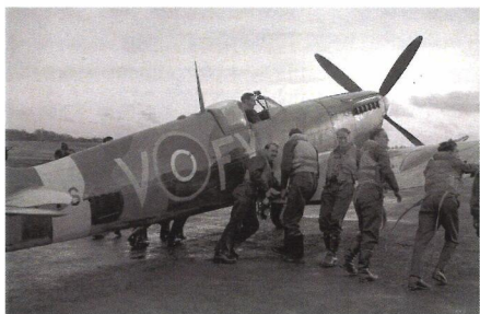
This British Spitfire has been polished with beeswax to reduce drag, increase speed, and reduce fuel usage.
