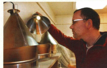
Bob Brown inspecting a wasp nest inside the mite extraction mechanism. A wasp nest is inserted into the funnel and a light/heat source at the top drives the mites down to the bottom, where they fall into a collecting tube.
