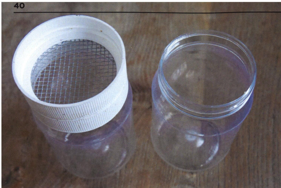
This alcohol wash container is made by Dr Medhat Nasr in Canada. It uses #8 wire galvanised mesh (the same as used in pollen traps). Lids are fused together with a soldering iron but can be plastic welded. Photo: Frank Lindsay.
