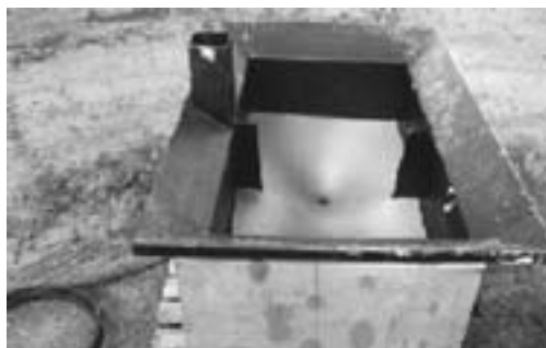
Photo 13. The vat operated by Sunderland Apiaries, Dubbo. Note the head space from the wax to the top of the walls. Note also the gas hose (bottom left) which is connected to the gas bottle located over three metres from the unit.
