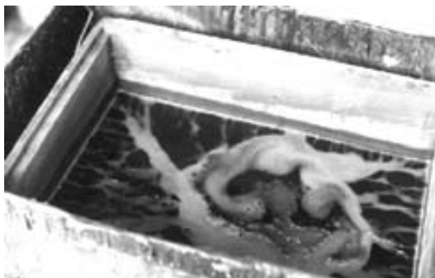
Photo 9 As the hot wax penetrates the timber and expels much of the moisture and air, the frothing reduces in intensity.
