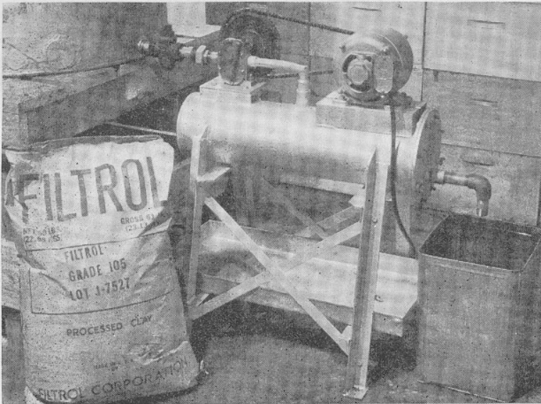
At the first stage of manufacture into comb foundation the crude wax is melted down in a steam-heated tank (upper left corner) and then in liquid form passed through a pressure filter in which diatomaceous earth is used as a filtration agent. After it has solidified it is processed in the Weed sheeting machine shown on page 193.
