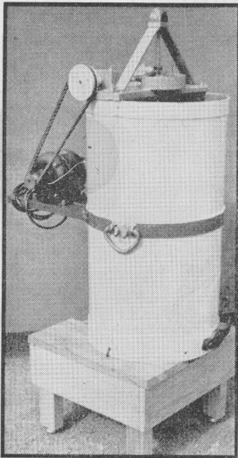
Honey stirrer fitted to a mixing tank which is a milk can set on a stand having ball castors.
