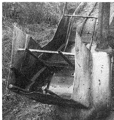
The level of liquid wax within the trough. Wire mesh over the upper guide rods supports block wax while it melts. The trough holds about three bags of wax. The tubular steel guide rods not only give a firmness to the flat iron, but force the hive boxes under the liquid wax as they are pushed, one behind the other, from the near end over to the drip tray.
